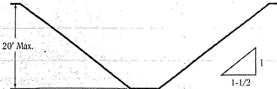
Figure 1. Excavations Made in Type C Soil
